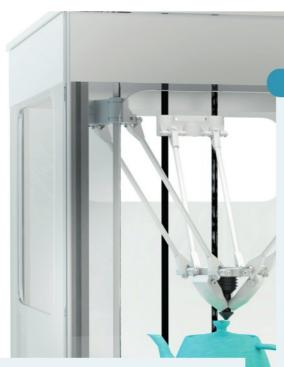
Additive manufacturing is a technique that uses 3D printers to build an object up bit by bit rather than taking a block of material and cutting bits away. Designers use vectors to create the 3D models which are then put through specialist software to render the object printable. → Exercise 1C Q11 Prior knowledge check
