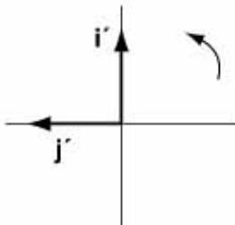
i.e. Rotation of  $90^\circ$  anticlockwise about  $(0, 0)$ .
