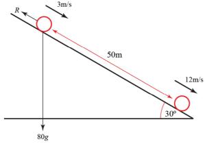
**a** Work done by resistive forces on the skier = change in total energy of the skier Loss in P.E. = mgh
