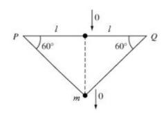
The modulus of elasticity of the spring is  $mg\sqrt{3}$ .
