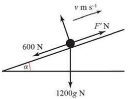
Let the speed of the car be  $u \text{ ms}^{-1}$ and the driving force of the engine have magnitude F'N.
