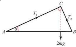
**a** The line of action of the weight must pass through *C* which is not above the centre of the rod.
