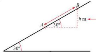
The change in the potential energy of *P* depends on the vertical distance it has moved. You find this using trigonometry.
