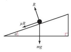
Let the normal reaction between the particle and the plane have magnitude *R* N
