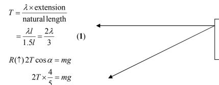
You find two equations in T and  $\lambda$  by resolving vertically and using Hooke's law. Eliminating T between the two equations gives  $\lambda$
