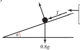
Initially the spring is in compression and the force of the spring on the particle is acting down the plane.
