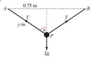
Let AP = y m and the angle AP makes with the vertical be  $\alpha$ . By trigonometry
