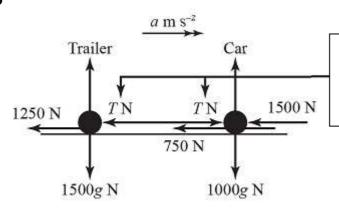
As the car brakes, the forces in the tow-bar are thrusts and act in the directions shown in this diagram. The forces in the tow-bar in **a** are tensions and act in the opposite directions to thrusts.
