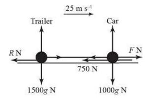
Let *F* N be the magnitude of the driving force produced by the engine of the car.
