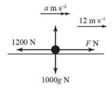
**a** Let *F* N be the magnitude of the driving force produced by the engine of the car.
