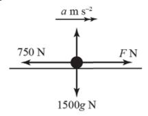
Let the acceleration of the lorry be  $a \text{ m s}^{-2}$  and the driving force of the engine have magnitude FN.
