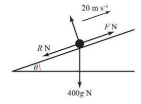
Let *F*N be the magnitude of the driving force produced by the engine.
