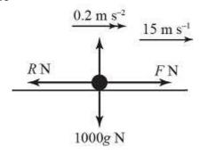
**a** Let *F* N be the magnitude of the driving force produced by the engine of the car.
