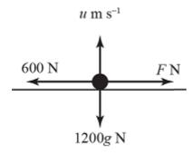
Let the speed of the car be  $u \text{ m s}^{-1}$  and the driving force of the engine have magnitude FN.
