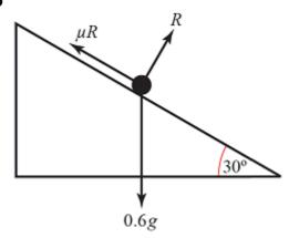
Let the normal reaction between the particle and the plane have magnitude R N.
