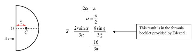
Centre of mass is on the axis of symmetry at a distance  $\frac{16}{3\pi}$  cm from the centre.
