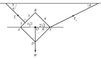
Origin *O* at centre of mass of framework. *AC* lies on *x*-axis. Resolve forces in *x* direction.
