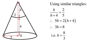
The centre of mass lies on the axis of symmetry. Let the centre of the base of the large cone be O.
