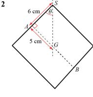
The diagram shows the equilibrium position with the centre of mass G below the point of suspension S.
