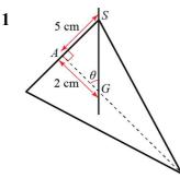
The diagram shows the equilibrium position with the centre of mass G, vertically below the point of suspension S.
