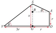
In equilibrium the centre of mass G lies below the point of suspension S. Let distance SG = x. O is the centre of the base of the cone and V is its vertex.
