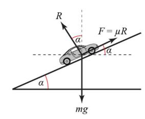
If the car is not to skid up or down the slope, the speed must remain between  $23.4 \text{ ms}^{-1}$  and  $77.4 \text{ ms}^{-1}$  (to 3 s.f.).
