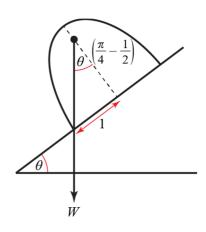
The solid is on the point of toppling when the plane is inclined at an angle of 74° (to the nearest whole degree) to the horizontal.
