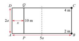
Treating the existing framework as a single object, taking the same axes as before and letting the centre of mass of the loaded framework including the rod PQ:
