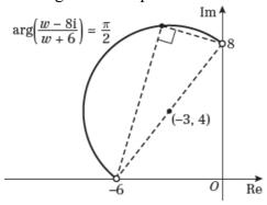
**b** The centre of this semicircle lies in the middle of the line connecting (-6,0) and (0,8), i.e. at (-3,4). The radius can be found be using Pythagoras Theorem:
