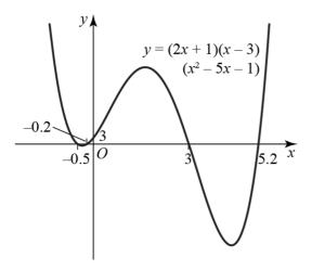
The solution corresponds to the section of the graph that is below the x-axis.
