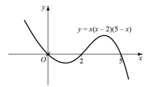
The solution corresponds to the section of the graph that is above the *x*-axis. So the solution in set notation is  $\{x: x < 0\} \cup \{x: 2 < x < 5\}$
