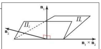
This diagram illustrates that the line of intersection of the planes  $\Pi_1$  and  $\Pi_2$  lies in the direction of  $\mathbf{n}_1 \times \mathbf{n}_2$ . In this case,  $4\mathbf{i} + 13\mathbf{j} + 25\mathbf{k} = -\mathbf{n}_1 \times \mathbf{n}_2$  and can be used as the direction of the line, as can any other multiple of this vector.
