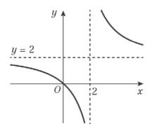
The curve crosses the axes at (0, 0). The horizontal asymptote is y = 2. The vertical asymptote is x = 2.
