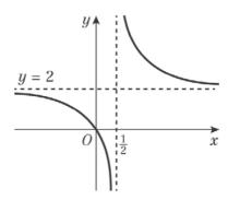
The curve crosses the axes at (0, 0). The horizontal asymptote is y = 2. The vertical asymptote is  $x = \frac{1}{2}$ . **2 f**  $f(\frac{1}{2}x)$  is a stretch with scale factor 2 in the *x*-direction.
