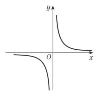
There are no intersections with the axes. The horizontal asymptote is y = 0. The vertical asymptote is x = 0.
