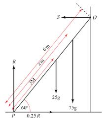
The maximum distance the builder can climb up the ladder before it slips is 2.46 m (3s.f.).
