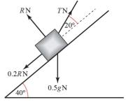
$T_{\text{MAX}}$  occurs when the particle is on the point of moving up the plane. At this point, limiting friction  $F = \mu R$  acts down the plane:
