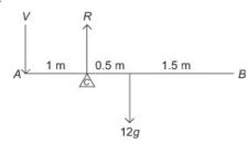
Suppose that the force required is V N acting vertically downwards at A. Taking moments about the pivot (C):
