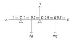
2 If the bar is about to tilt about C then the reaction at D is zero. Let the distance AE = x m
