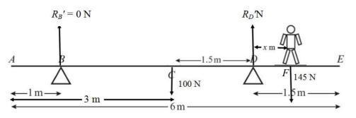
When the plank is on the point of tilting, the new reaction force at support B,  $R'_B = 0$  N and plank is again in equilibrium. The child stands a distance x m from support D.
