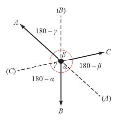
Since the body is in equilibrium, the forces A, B and C form a closed triangle as shown below:
