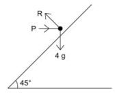
**11 a** Let the normal reaction between the particle P and the plane be R N. Let the tension in the string be T N.
