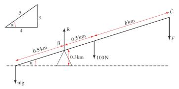
To lift the mass, total clockwise moments about *B* must exceed total anticlockwise moments about *B*:  $(F \times 1.5k \cos \alpha) + (100 \times 0.5k \cos \alpha) > mg \times 0.5k \cos \alpha$
